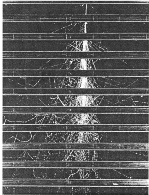
Fig. 2. A cloud chamber photograph (MIT cosmic ray group) of a particle traversing a series of brass plates demonstrates that a single particle can indeed give rise to multiple secondary particles. (Reproduced with permission of the McGraw-Hill Companies from Ref. 2, p. 96.)
