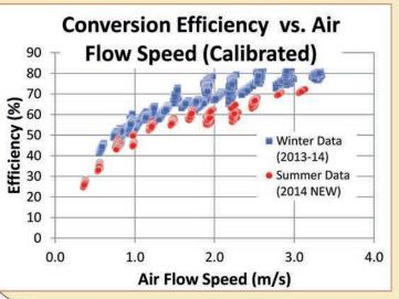
The conversion efficiency approaches 80% as we increase the flow speed to 3.0 m/s
