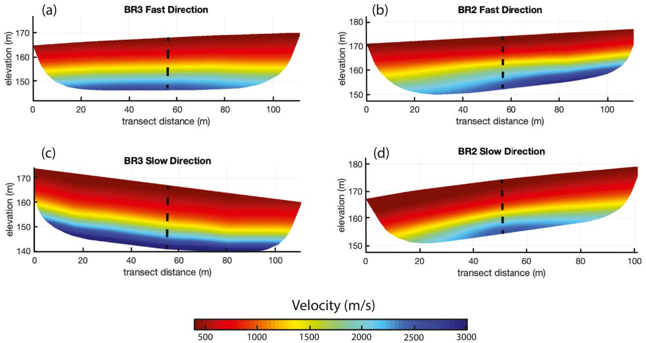
**Figure 4.** Tomograms used to calculate  $A_v$  colored for velocity. Note that seismic lines from the same site intersect halfway along their transects. The points of intersection are denoted by dashed black lines. Also note that the middles of intersecting tomograms from (a) and (c) are compared to calculate the blue curve while those from (b) and (d) are compared to calculate the red curve in Figure 5b.
