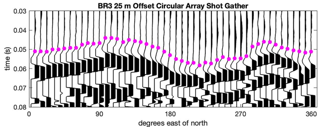
**Figure 2.** Example of a shot gather from the 25 m offset circular array at the BR3 site with first arrival picks marked as purple dots. Note the sinusoidal pattern in first arrival times and the high signal-to-noise ratio.
