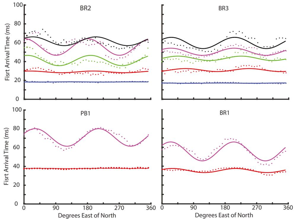
**Figure 3.** First arrival times and fitted cosine function from each survey site. First arrivals and fits are colored according to the radius of the survey with blue, red, green, purple, and black corresponding to 6.25, 12.5, 18.75, 25, and 37.5 m offsets respectively.  $R^2$  values for fits can be found in Table 1.
